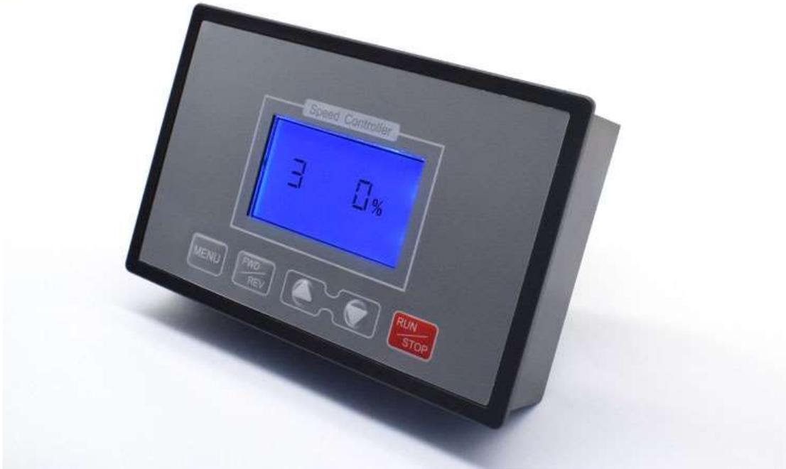
Speed limit setting Press the **MENU button 5 times** to enter the function 4 key surface Press the plus and minus keys to set the size value Press RUN/STOP to save and exit.
