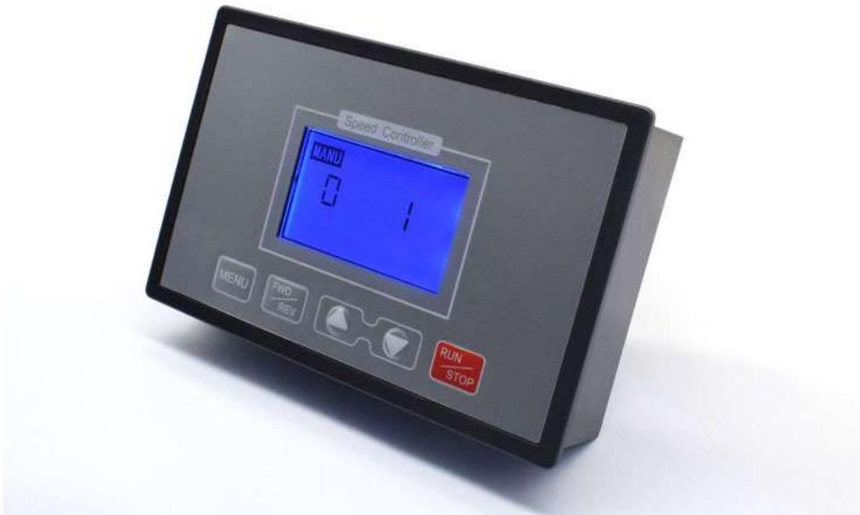
Slow start time setting Press the **MENU button 2 times** to enter the function 1 setting key surface Press the plus and minus buttons to set the time Press RUN/STOP to save and exit (10 is 1 second, 100 is 10 seconds)
