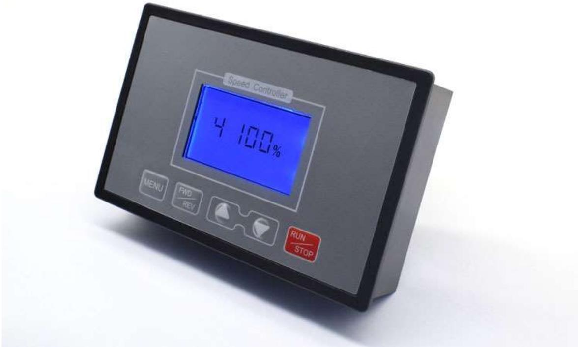
Set acceleration and deceleration value Press the **MENU key 6 times** to enter the function 5 key surface Press the plus and minus keys to switch Press RUN/STOP to save and exit
