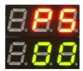
Pressing **SET** again causes the value to flash and allows the value to be changed.
