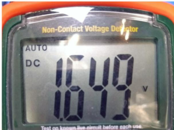
Hook up a multimeter to the Vout pin of the board (positive/red lead to Vout, ground/black lead to board GND) and you should see about 1.65 volts DC output. Try setting `dac.value` to other numbers like 0 or 65535 to see how the voltage changes.
