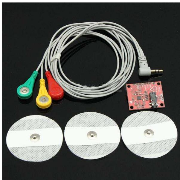
AD8232 Adopts an operational amplifier that is without using constraint to build a three pole low pass filter, eliminating extra noises
